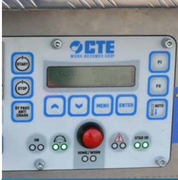
DIAGNOSTIC TOOL INTEGRATED IN THE CONTROL PANEL
