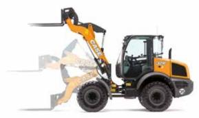
Z-bar is the most versatile linkage type. It offers more breakout force thanks to the 2 lifting cylinders and a higher dump height.
