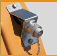
A 14-pin Front Electric system provides four independent activation systems that can be called up with the touch of a button on the control handles.
