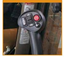
A standard thumb wheel controls a fully proportional auxiliary hydraulic system, giving the operator pinpoint control of hydraulic flow in either direction. It has detents in both directions for continuous operation, providing less fatigue and more precision results.
