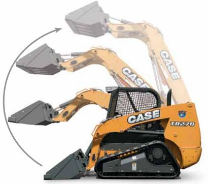
**Vertical-lift** machines are engineered for lift-and-carry and truck loading. The geometry of the dual-arm allows the load to rise directly up providing maximum reach at full height—ideal for reaching over the side and into the middle of high-side trucks.
