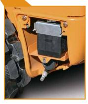
The convenient side panel gives access to the battery, remote oil drain and engine oil filter. There is also direct access to the oil pan under the machine for faster oil drainage.
